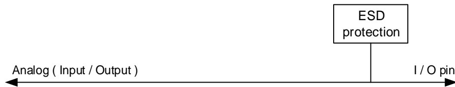
Figure 7-4. Basic structure of Analog configuration
