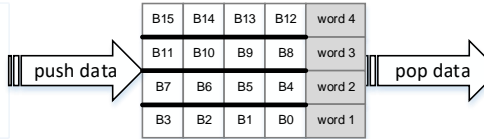
Figure 10-4. Data packing/unpacking when PWIDTH = '00'
